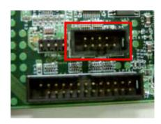
LPTA1: Parallel Connector (26 Pin 2.00mm Pitch Header)
